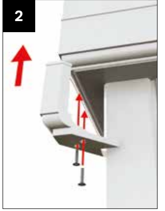
WITH COLUMNS - LPCS090 (only) or LPCL090 Whilst ensuring that the corner remains located in position, screw fix using self drilling screws CRN007.
