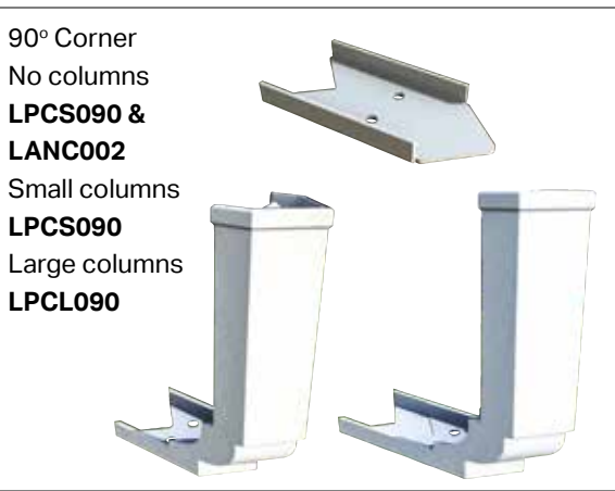
WITH COLUMNS - LPCS090 (only) or LPCL090 Whilst ensuring that the corner remains located in position, screw fix using self drilling screws CRN007.
