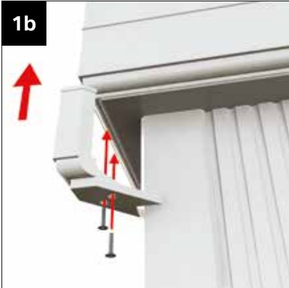
WITH COLUMNS - LPCS090 (only) or LPCL090 Whilst ensuring that the corner remains located in position, screw fix using self drilling screws CRN007.
