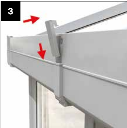
3 Slide the bracket into place ensuring bracket cleats slot into the top Cornice section.
